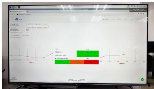
A palm-sized computer linked to a monitor helps to display WBGT readings at regular intervals.
