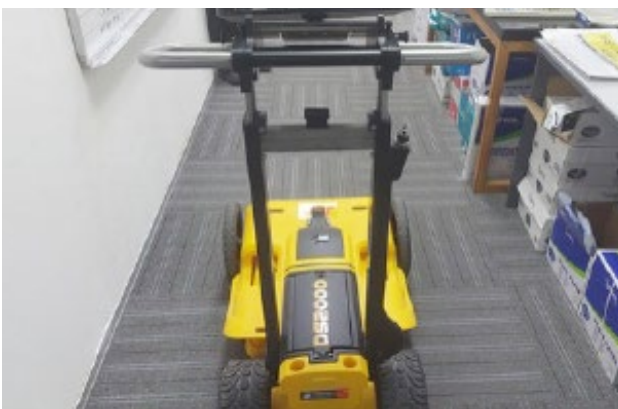
By adopting the Leica DS2000 utility detection radar's advanced ground-penetration technology, OKP is able to accurately detect underground utilities.
