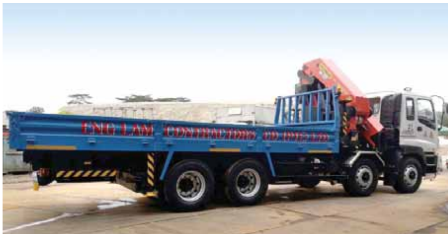
Newly purchased lorry crane used to support OKP projects.
