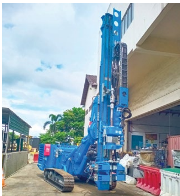
A newly purchased drilling rig for jet grouting.
