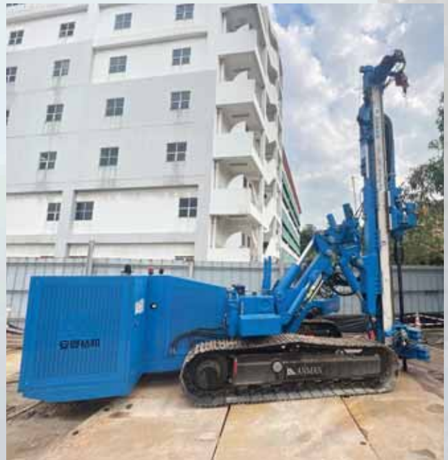
A newly purchase jet grouting machine to support OKP's projects.
